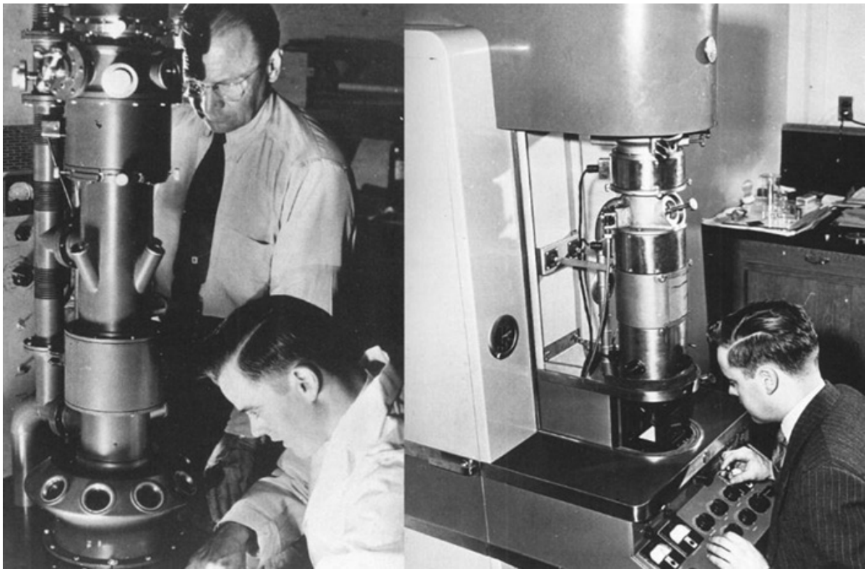
The photo on the left shows the first commercial electron microscope (the EM) from Radio Corporation of America (RCA), in 1940, operated by James Hillier with Alexander Zworykin, RCA's research chief and instigator of the EM project, looking on. This was followed in 1943 by the RCA "universal" EM, the EMU (right), which was capable of both imaging and diffraction. The EM, invented in 1931, first made it theoretically possible to see viruses for the first time. Viruses are not visible with a normal light microscope, but the EM uses fast electrons, which have a much smaller wavelength than visible light, to depict a sample's surface. And since a microscope's resolution is limited by the wavelength, a much higher resolution can be achieved with an EM (currently approximately 0.1 Nanometer = billionth of a meter) than with a light microscope (approximately 0.2 micrometers = millionth of a meter). Source: James Hillier 1915 - 2006: Contributions to Electron Microscopy, www.microscopy.org
