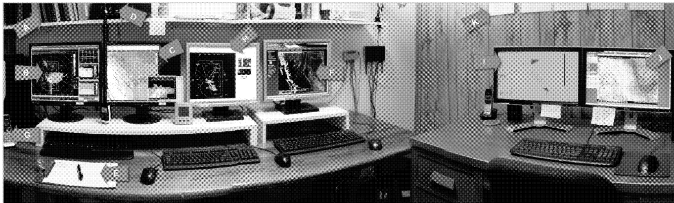
Figure 22. The configuration of the Operations Room. Equipment includes (A) reference manuals, (B) TITAN displays, (C) CIDD, (D) VHF radio for communications with aircraft, (E) radar log, (F) internet data displays, (G) telephone, (H) AirLink display, (I and J) forecasting/nowcasting support displays, and (K) radio and radar licenses. (WMI wide-angle photograph by Daniel Gilbert.)
