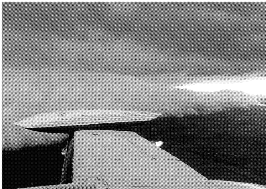
Figure 7. A wing-tip generator on Hailstop 4 produces ice nuclei in the inflow region of a thunderstorm west of Sylvan Lake on 23 June 2016, at 8:44 PM. (WMI photograph by Richard Oxlade.)
