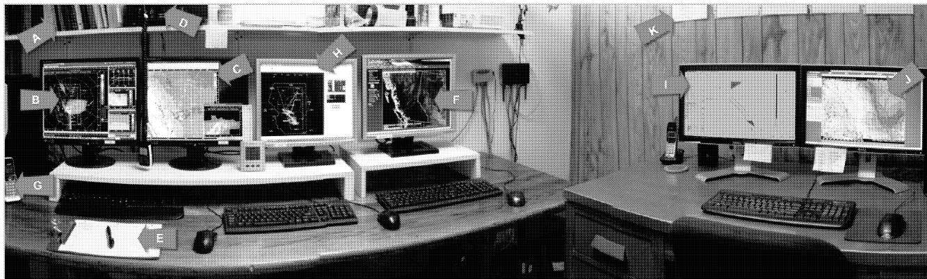
Fig. 21. The configuration of the Operations Room. Equipment includes (A) reference manuals, (B) TITAN displays, (C) CIDD, (D) VHF radio for communications with aircraft, (E) radar log, (F) internet data displays, (G) telephone, (H) AirLink display, (I and J) forecasting/nowcasting support displays, and (K) radio and radar licenses. (WMI wide-angle photograph by Daniel Gilbert.)
