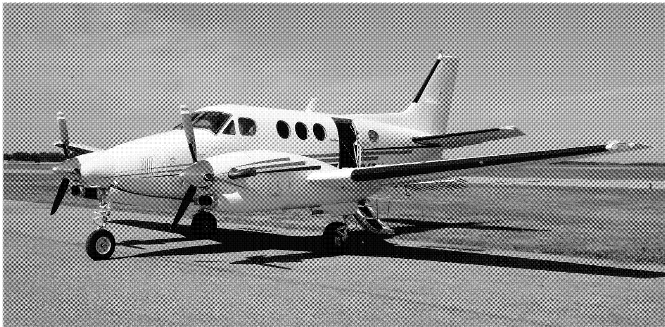
Fig. 19. A King Air model C90, Hailstop 1, awaits the development of convective weather on the morning of 2 July 2015. Racks of burn-in-place pyrotechnics are visible aft of the near wing. (Photograph courtesy of Terry Krauss.)
