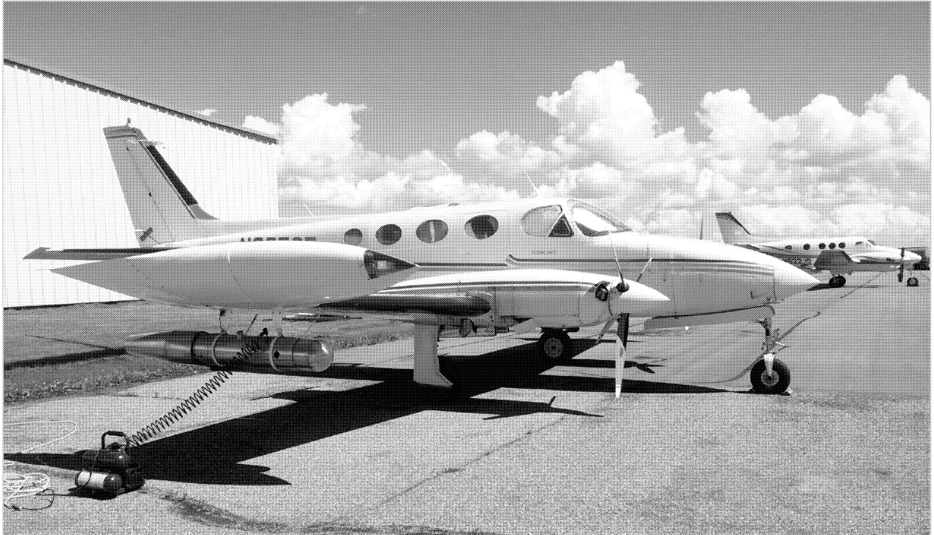
Fig. 19. Hailstop 4, a Cessna 340A seeding aircraft is shown on the ramp in Red Deer. Notable on the aircraft (and absent from the turboprop aircraft such as Hailstop 3, seen in the background) are the wing-tip ice nucleus generators, the silver torpedo-like appurtenances below the wing-tip fuel tanks. The photograph was taken just prior to the daily weather briefing, during preflight inspection. The compressor is used to fill a pressure tank in the front of the generator that provides the flow of seeding solution to the rear, where it is burned. (WMI photograph by L.J. Dunn.)
