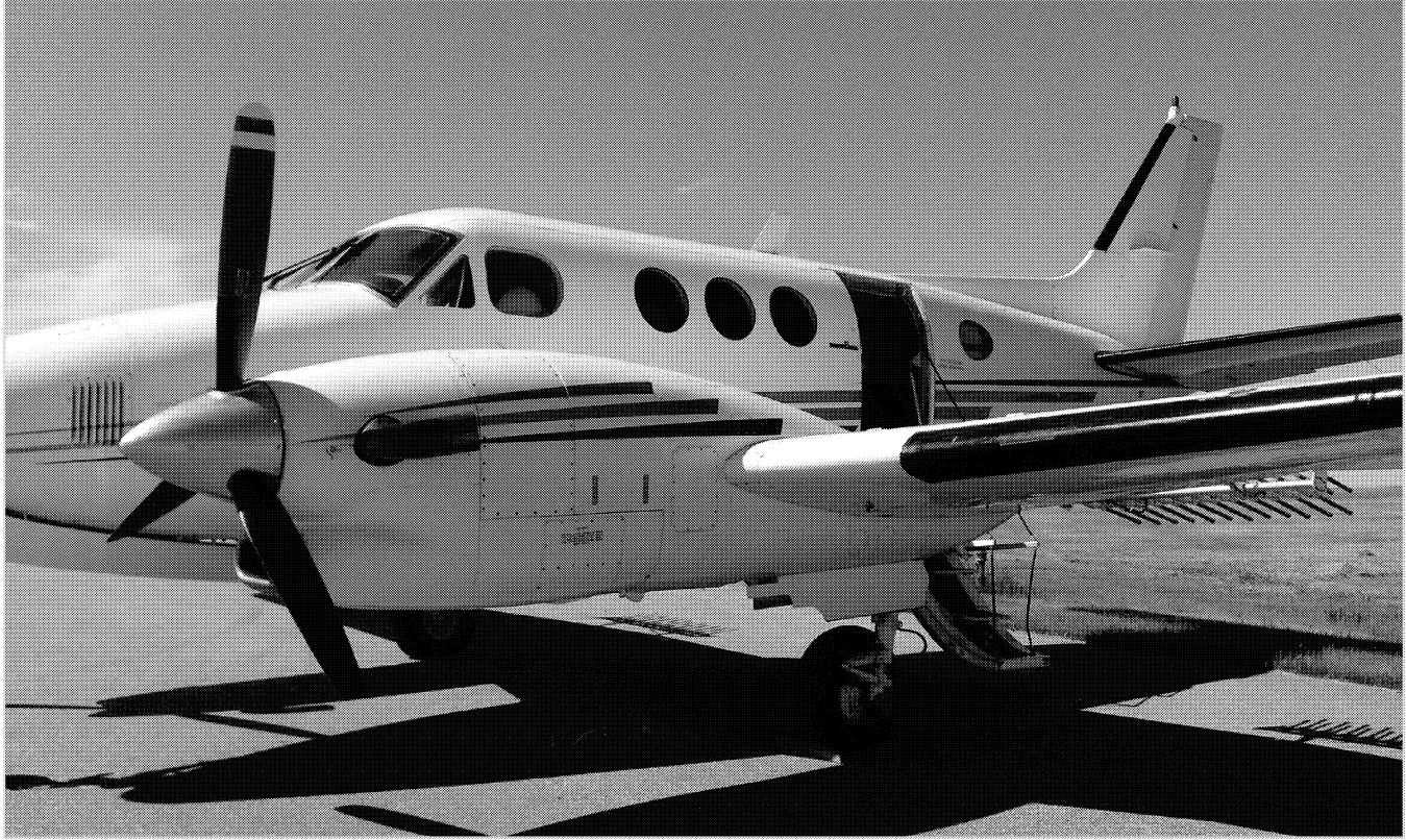
Fig. 18. Hailstop 1, one of three King Air C90 aircraft on project, sits on the ramp at the Olds-Didsbury Airport, awaiting visitors attending an accredited insurance industry tour, on June 23, 2014. A “double-rack” of burn-in-place cloud seeding pyrotechnics is clearly visible aft of the engine on the near wing. The racks for smaller, ejectable flares mounted on the aircraft belly are not visible. (WMI photograph by Adam Brainard.)
