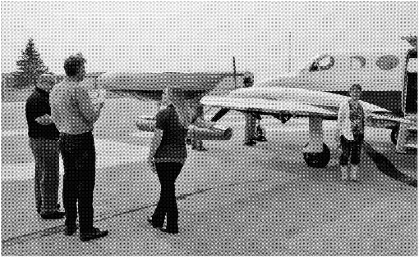
Fig. 20. Captain Jenelle Newman (hand on wing-tip ice nucleus generator) explains the seeding equipment on Hailstop 4 to some of the participants in the August 16 th , 2018 continuing education tour and seminar at the Olds-Didsbury Airport, while another attendee waits at the base of the aircraft door her turn to check out the seeding aircraft interior. (WMI photograph by Adam Brainard.)
