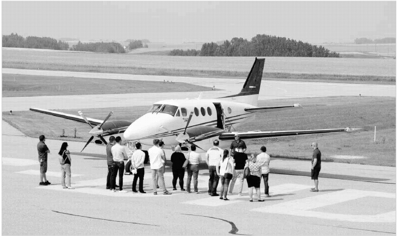
Fig. 25. A King Air model C90, Hailstop 3, sits on the Olds-Didsbury Airport ramp on August 9 th , while Captain Joel Zimmer (in blue, facing camera) introduces the tour-goers to how the aircraft is used on the project. Racks of burn-in-place pyrotechnics are visible aft of the near wing. (WMI photograph by Adam Brainard.)
