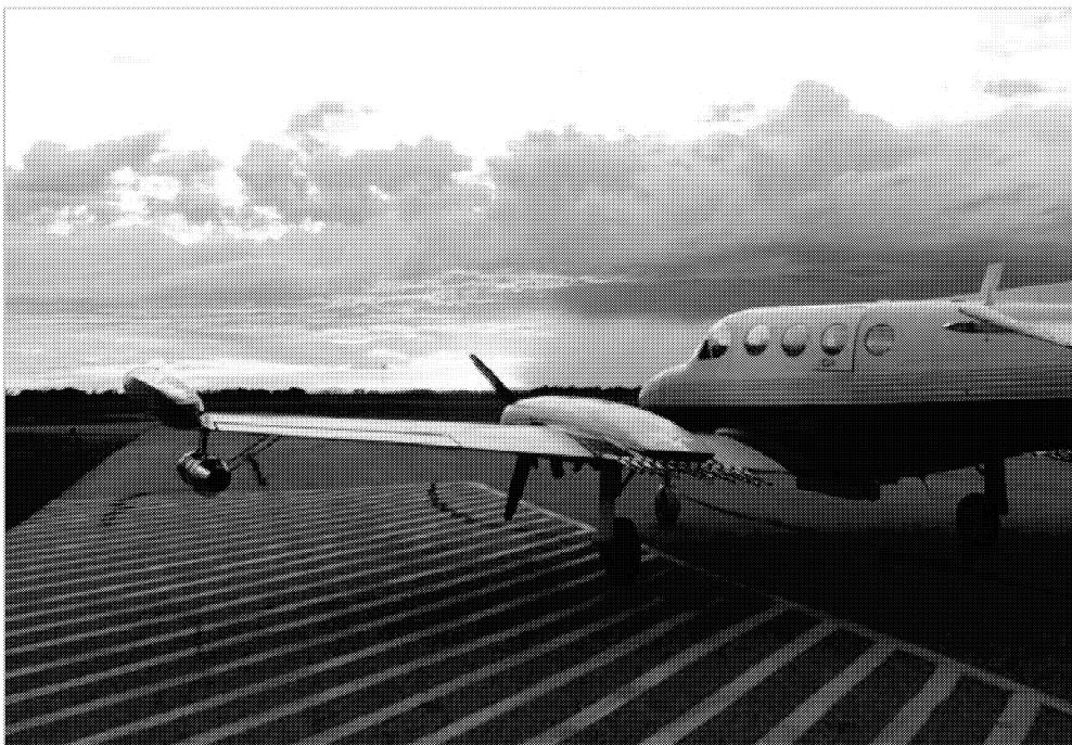
Fig. 6. Hailstop 4 sits on the ramp at sunset on July 6 th , just after landing from a seeding mission that ranged from Olds, to Sundre, and then northeast toward Red Deer. Careful examination reveals the remnants of expended burn-in-place flares, still attached to the left wing rack. (WMI photograph by Trevor Black.)
