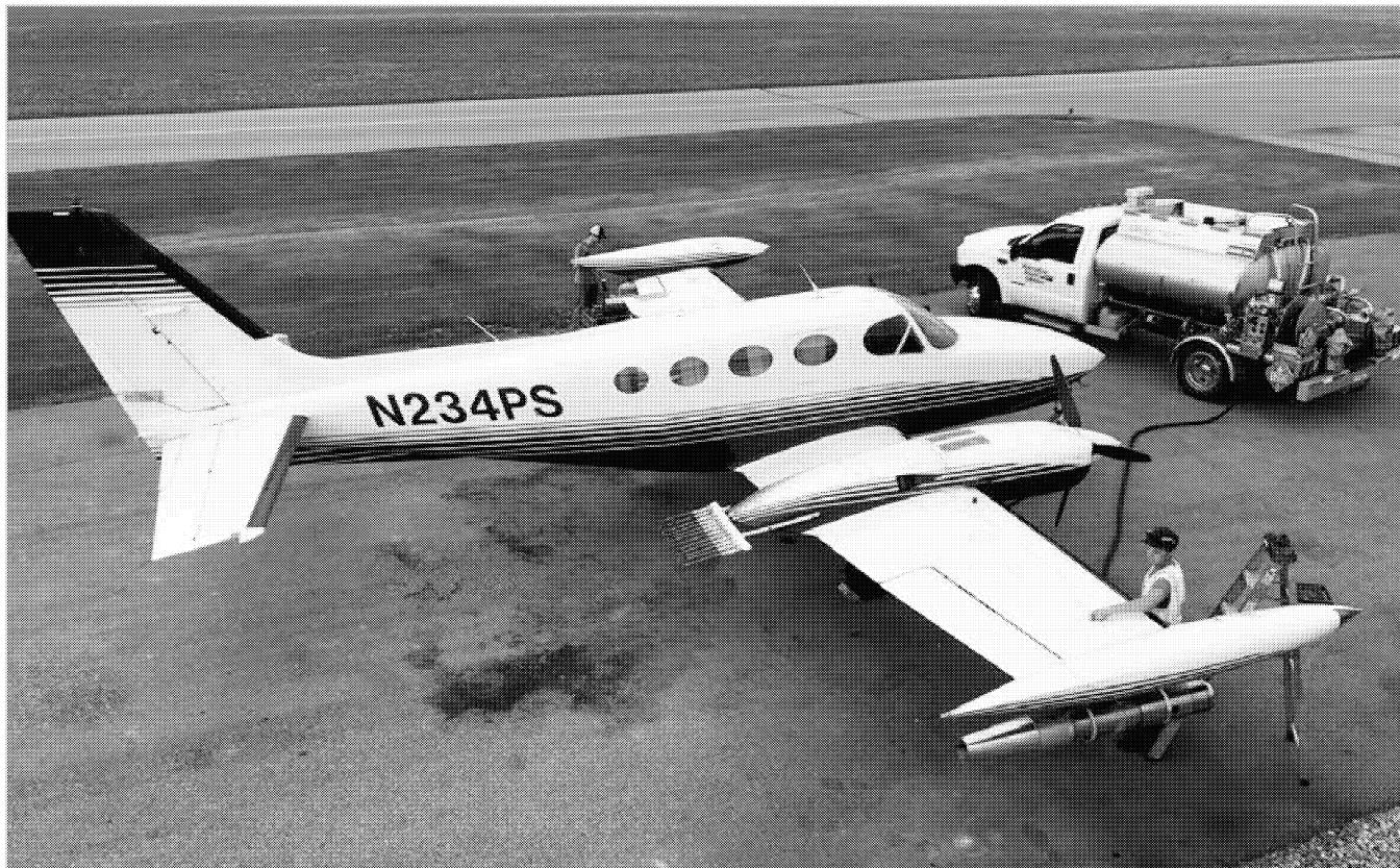
Fig. 26. A Cessna model 340A, Hailstop 2, rests on the ramp at the Springbank Airport, after the season's first day on which all five Hailstop aircraft flew, June 9 th . While the Springbank Aero crew refuels the aircraft, co-pilot Matt Burrus refills seeding solution for the far ice nucleus generator. (WMI photograph by Brian Kindrat.)
