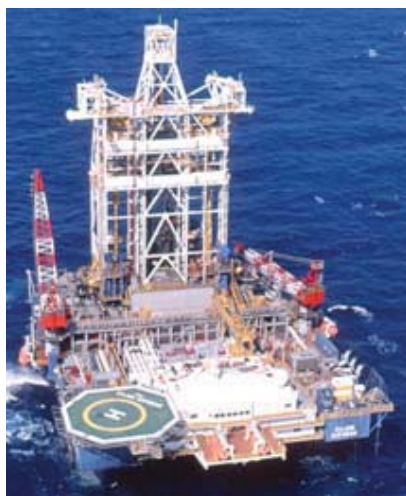
Figure 39: The Cajun Express deep water drilling rig. At 106x70m and with up to 10.6 km (35kft) of pipe down to a pocket of high pressure oil and natural gas, these off shore rigs are analogous to a floating geoengineering platform (Transocean image, http://www.deepwater.com/fw/main/Cajun-Express-52C17.html ).
