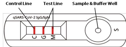
When a correct volume of test specimen is dispensed into the sample well of the test cassette, the specimen migrates by capillary action along the cassette. The anti-SARS-CoV-2 virus IgG, if present in the specimen, will bind to the SARS-CoV-2 conjugates. If IgG is present in the specimen, the immunocomplex will then be captured by the anti-human IgG line, forming a burgundy colored G Line, indicating a SARS-CoV-2 virus IgG positive test result.
