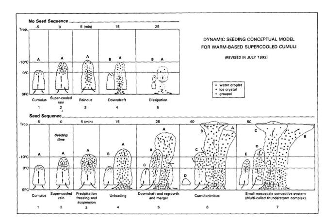
Figure 1: Diagrammatic illustration of the dynamic seeding conceptual model for warm-based supercooled cumuli. Revised as of July 1992. [From Rosenfeld and Woodley, 1993.]
